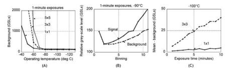
Fig. 3. (A) Mean gray scale level (GSL) for different operating temperatures and hardware binning levels for 1-minute exposures. (B) Relative GSLs for signal from a geranium leaf and background with no object as a function of hardware binning level. (C) Mean GSLs as a function of exposure time for two different hardware binning levels.
