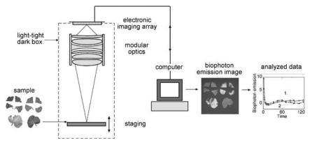
Fig. 1. Schematic of biophoton imaging system.
